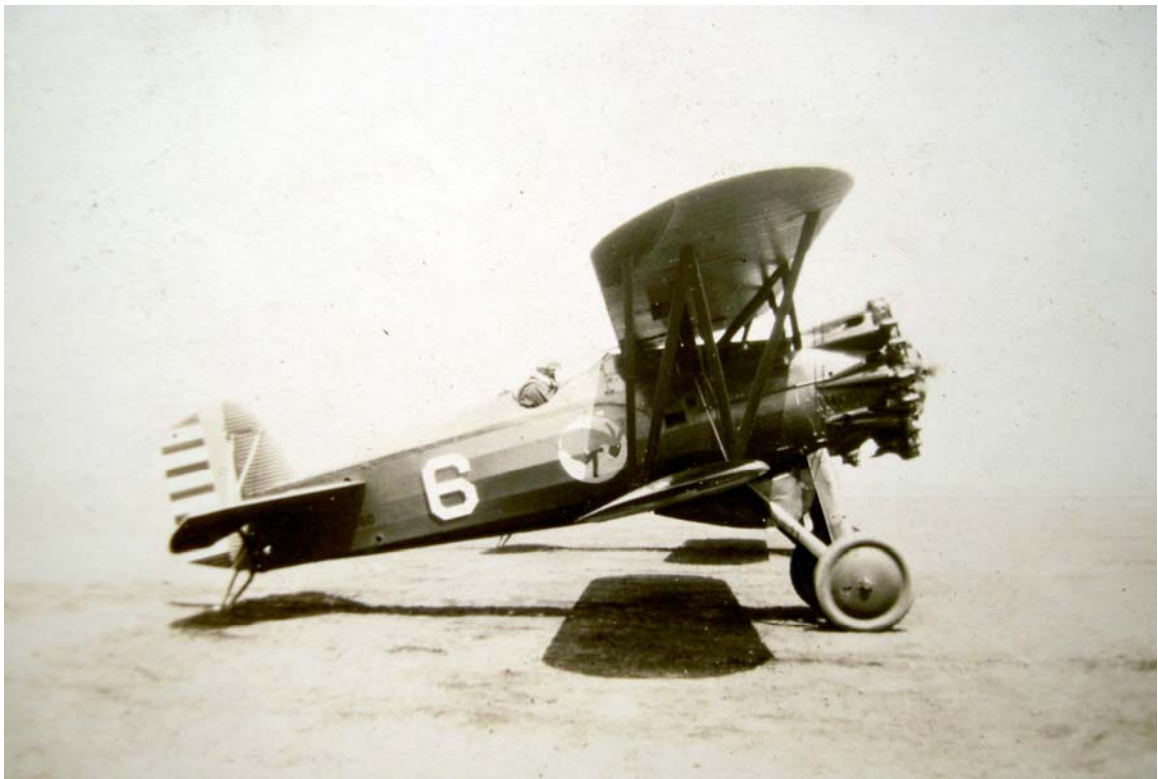
March Field-based Boeing P-12s of the U.S. Army's famed 95th "Kicking Mule" Aero Squadron (17th Pursuit Group) with 50-gallon auxiliary belly tanks. Powered by the 450 hp P&W "Wasp," top speed was 190 mph, cruise 167 mph. The nimble, high-performance P-12 / F4B series was a major leap forward compared to earlier designs. Milo Burcham, whose Boeing 100 was a civilianized version of this aircraft, is said to be the first airshow pilot capable of performing sustained "knife-edge" flight due to the tremendous power and performance of this aircraft. Navy tests revealed the stream-lined cylinder fairings on the early F4B-1 / P-12 aircraft actually impeded cooling and when removed resulted in a 5 mph speed increase! Perhaps ironically, Burcham's Boeing 100 survived the years and was restored to flying condition as a P-12 of the 95th, sporting the numeral 3 on its side panel. Russ Gerow photo, Long Beach, 1929. R.T. Gerow Collection
