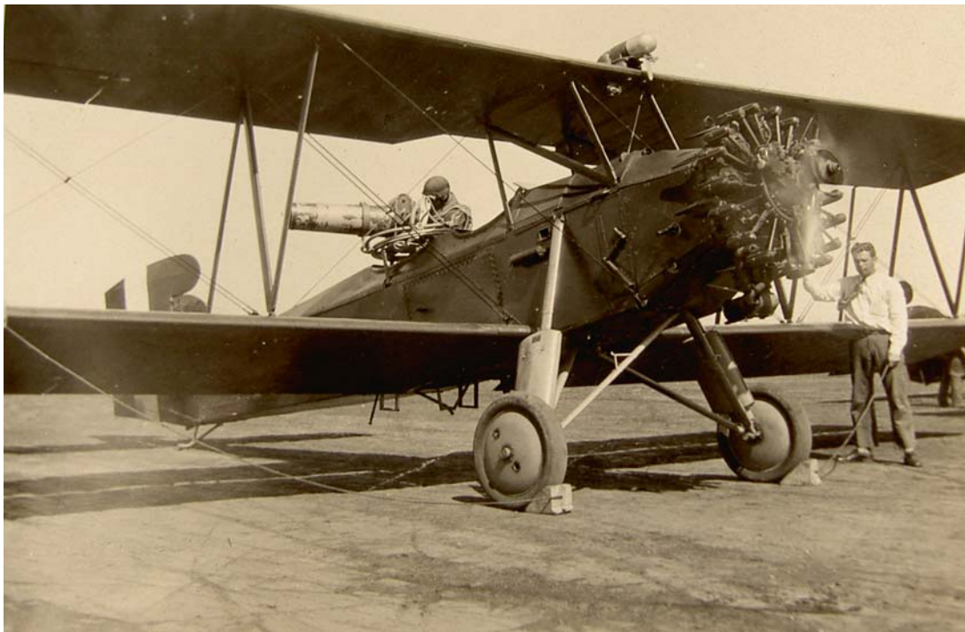
Powered by the same engine as the "Spirit of St. Louis," the reliable Wright J-5 "Whirlwind" produced 220 hp at 2,000 rpm, giving the Fledgling a top speed of 109 mph.
