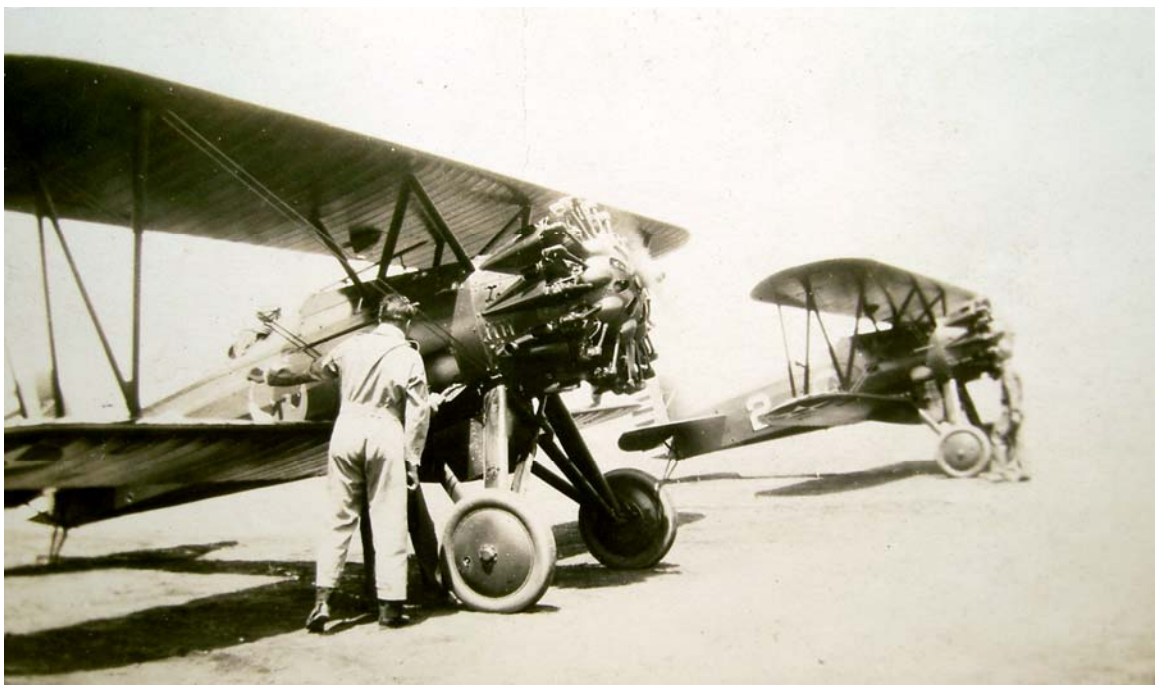
March Field-based Boeing P-12s of the U.S. Army's famed 95th "Kicking Mule" Aero Squadron (17th Pursuit Group) with 50-gallon auxiliary belly tanks. Powered by the 450 hp P&W "Wasp," top speed was 190 mph, cruise 167 mph. The nimble, high-performance P-12 / F4B series was a major leap forward compared to earlier designs. Milo Burcham, whose Boeing 100 was a civilianized version of this aircraft, is said to be the first airshow pilot capable of performing sustained "knife-edge" flight due to the tremendous power and performance of this aircraft. Navy tests revealed the stream-lined cylinder fairings on the early F4B-1 / P-12 aircraft actually impeded cooling and when removed resulted in a 5 mph speed increase! Perhaps ironically, Burcham's Boeing 100 survived the years and was restored to flying condition as a P-12 of the 95th, sporting the numeral 3 on its side panel. Russ Gerow photo, Long Beach, 1929. R.T. Gerow Collection
