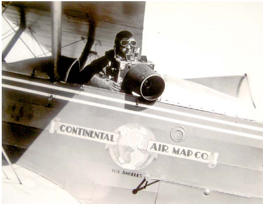
Russ Gerow demonstrates the Fairchild K-4 aerial camera mounted for oblique photography in the middle crew station of Continental Air Map's Douglas M-4. With a 1924 military sticker price of $2,628.62, the 46-lb. K-3 was the first camera to solve the vexing inter-lens shutter and film-spacing-system problems that plagued earlier aerial cameras. Offering selectable shutter speeds of 1/50th, 1/100th and 1/150th/sec, its standard 7" x 9-1/8" film yielded 115 exposures per 75-foot roll of film. Introduced in 1925, the $3,516 K-4 camera was basically a K-3 with an 8-inch lens cone and a heftier price tag. Photo taken at Long Beach, c. 1930-31, photographer unknown. Russell T. Gerow Collection
