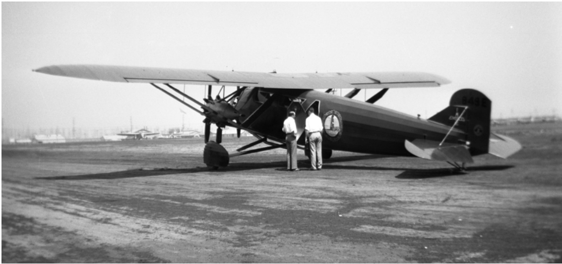
EMSCO B-2 "Challenger" designed by Charles F. Rocheville. This photo, taken by Russ Gerow, possibly captures the roll out of this aircraft. Balding man on left is probably Thomas D. "Jack" Reid. A close look at the rudder reveals the number 849E which was subsequently registered X849E on May 17, 1929. The first official EMSCO aircraft, 849E was powered by three 170 hp Curtiss "Challenger" engines, hence the aircraft's name. It was advertised as being able to take off with a full load with any two engines operating. In January 1930, the aircraft was converted to a twin-engine configuration using 300 hp Wright J-6s and redesignated EMSCO B-5 "Whirlwind." After a 7,000-mile promotional junket to EMSCO's various holdings around the country, NC849E was flown in August 1933 to its new owner in Guatemala City, where its ultimate fate remains a mystery. R.T. Gerow Collection.
