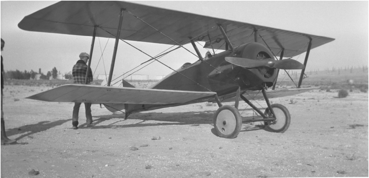
In evidence are the handsome lines of the 1917 Thomas-Morse S4C fighter trainer that Russ Gerow refurbished in his spare time as an auto and truck mechanic at the Ford Garage in Taft. Dick Kerr, co-owner of Continental Air Map and a fellow "Tommy" pilot, hired Russ as mechanic for Continental partly on the basis of this project. Powered by a Rhone 9C rotary engine of 80 hp, one wonders how the ship might have performed adapted to the beefier 160 hp Gnome Monosoupape. Note oil derricks and storage tanks in background. Photographer unknown, Taft, c. 1925-26. Russell T. Gerow Collection
