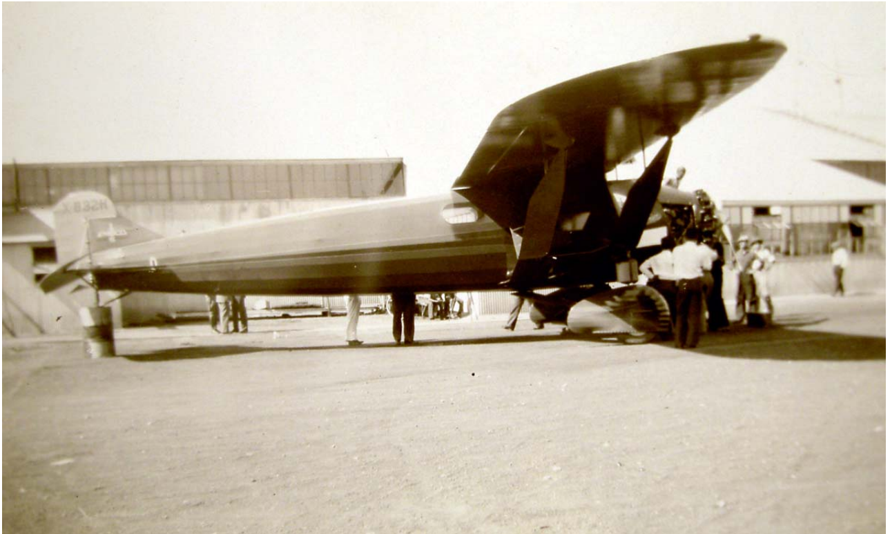
The second EMSCO aircraft (X-832H) was the first of the B-3 series, seen here readying for a test flight at Long Beach. In lower photo, note glare reflecting off immaculate finish for which EMSCO aircraft were famous. Russ Gerow's note on this picture reads: "Jack Reid's 'Death Ship.' This ship lifted over 6,000 lbs gas and oil with a single 300 h.p. engine. Flown by Reid and Bronte at Long Beach Airport. Reid was killed in ship at Cleveland. Emsco aircraft designed by Chas. Rocheville." Reid, an EMSCO employee and old Navy friend of Rocheville, set a new world's solo endurance record with this aircraft on Aug. 21, 1929, but fell asleep and crashed 38 hours 40 minutes into the flight. In a snafu emblematic of EMSCO's chronic hard luck, Reid was actually airborne hours earlier waiting for the delayed official timing of the flight to begin. Photo Russ Gerow, Long Beach Airport, 1929. Russell T. Gerow Collection
