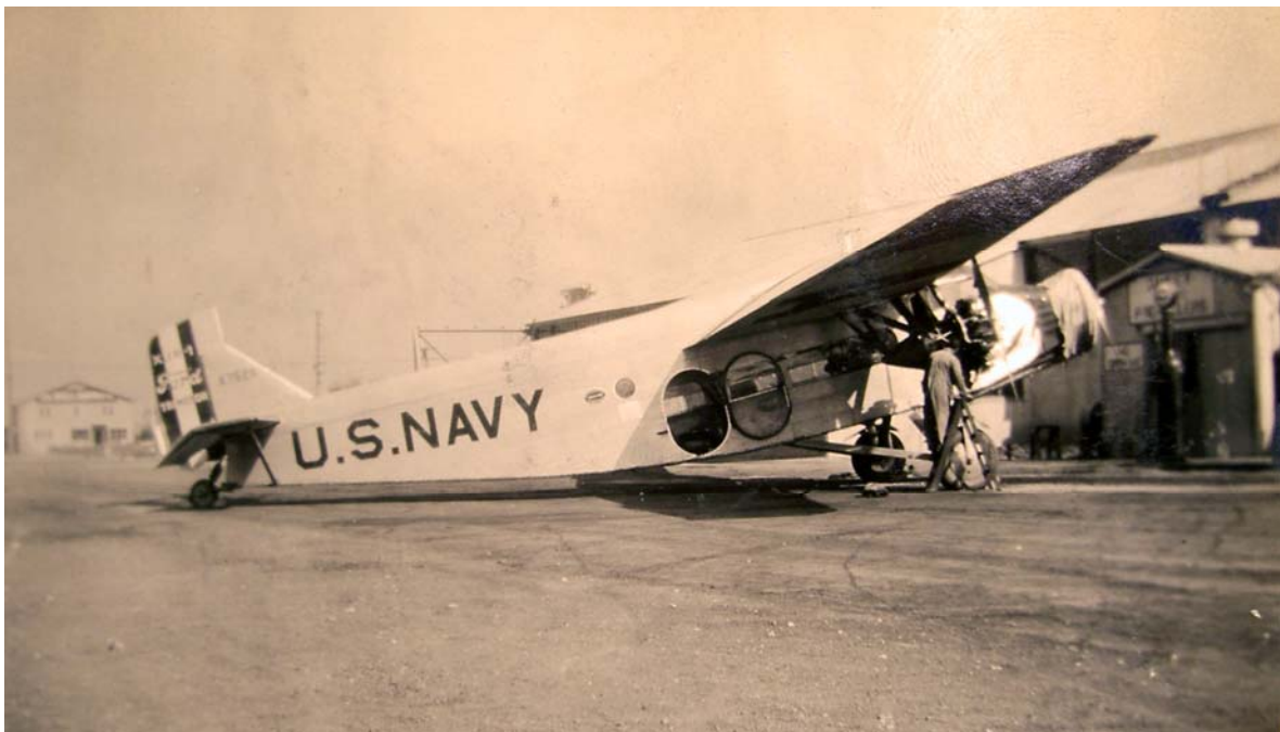
Ford XJR-1 Tri-motor (A-7526) powered by three 200 hp Wright J-4 engines. In 1928-29, according to www.dmairfield.com , this airplane flew semi-annual shuttles between its home field at Anacostia, Washington, DC and San Diego, CA, headquarters of the 11th Naval District. This photo, taken by Russ Gerow at Naval Reserve Aviation Base-Long Beach during this time period, shows A-7526 undergoing what appears to be routine maintenance. NRAB-LB was the terminus for military and government brass visiting the Battle Fleet anchored off San Pedro. The last time this aircraft landed for its customary fuel stop at Tucson was on June 19, 1929. A-7526 was flown on that occasion by famed Naval aviator D.W. "Tommy" Tomlinson carrying the Assistant Secretary of the Navy as his only passenger. R.T. Gerow Collection
