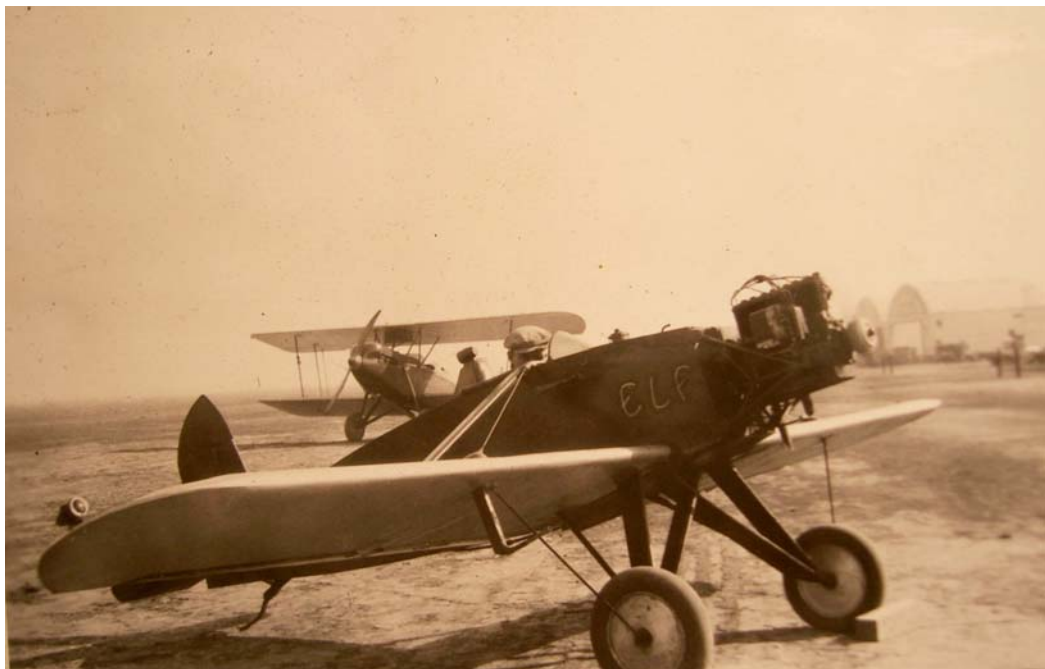
Long Beach aircraft designer Donald Smith running up his speedy home-built "Elf." According to Russ Gerow, this little ship was good for 140 mph, powered by a 27 hp four-cylinder Henderson motorcycle engine. Note slight forward stick has lifted the tail a few inches off the ground. The pictorial "Daily Magazine" page of the August 13, 1928 Oakland Tribune ran an AP publicity photo of Donald Smith and "Elf" alongside Charles Rocheville and his Albatross B1 as "The David and Goliath of Planes at Long Beach Airport." Russ Gerow photo, Long Beach flight line, 1928. R.T. Gerow Collection
