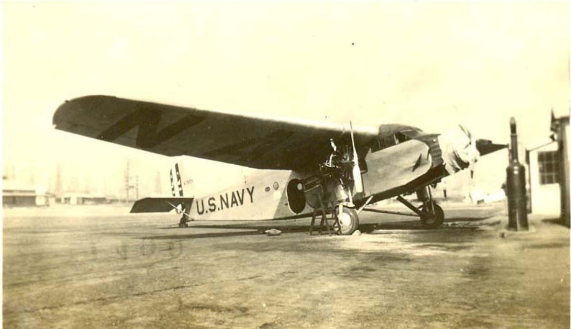
Ford XJR-1 Tri-motor (A-7526) powered by three 200 hp Wright J-4 engines. In 1928-29, according to www.dmairfield.com , this airplane flew semi-annual shuttles between its home field at Anacostia, Washington, DC and San Diego, CA, headquarters of the 11th Naval District. This photo, taken by Russ Gerow at Naval Reserve Aviation Base-Long Beach during this time period, shows A-7526 undergoing what appears to be routine maintenance. NRAB-LB was the terminus for military and government brass visiting the Battle Fleet anchored off San Pedro. The last time this aircraft landed for its customary fuel stop at Tucson was on June 19, 1929. A-7526 was flown on that occasion by famed Naval aviator D.W. "Tommy" Tomlinson carrying the Assistant Secretary of the Navy as his only passenger. R.T. Gerow Collection
