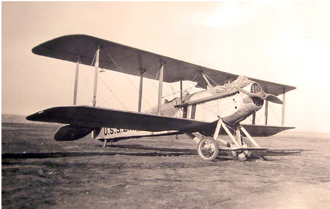
A significant aircraft in Naval aviation history, the 1917 Lewis & Vought VE-7 "Bluebird," despite its curiously non-belligerent nom de guerre , was the Navy's first frontline fighter. Serving in a number of roles, it was also the first US Navy aircraft to take off from the first US Navy aircraft carrier, USS Langley (CV-1) on October 17, 1922. Powered by a 185 hp Wright-Hispano Suiza E-2, the 106 mph VE-7 remained in service until 1928, when Langley's last three examples, including the above, were retired. Notice "Langley Stripe" between exhaust pipe and bottom wing. Designed by Chauncey M. Vought, the SPAD-like features of the VE-7 are obvious, but the Sopwith Camel-style vertical stabilizer is hidden in this view! Note experimental "fiddle bridge" arrestor hooks attached to landing gear to guide the landing aircraft along the ship's deck, so named because the arrangement suggested the stringing of a violin. This VE-7 was among the earliest Naval aircraft capable of shipboard landing. In 1922, the company became Chance Vought, originator of the famous Corsair biplane family of the 1920s and the even more famous F4U series, arguably the finest piston-engine shipboard fighter of WWII and the Korean War. Russ Gerow Photo, Long Beach, 1928. R.T. Gerow Collection
