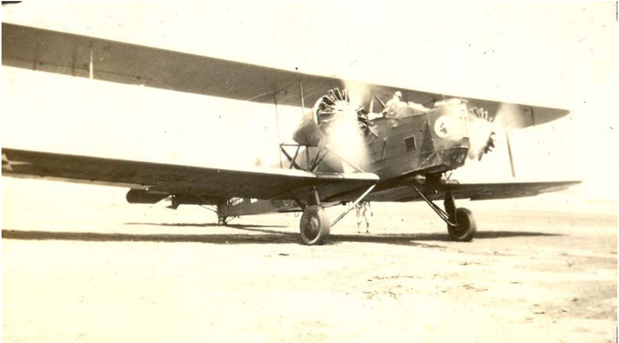
Two views of Keystone LB-7 (28-391) of the Army's 11th Bombardment Squadron based at Rockwell Field, San Diego. Powered by two 525 hp Pratt & Whitney R-1690-3 Hornet radials, top speed was 114 mph. A total of 16 LB-7s were delivered to the Army Air Corps, but they rapidly became obsolete and were removed from service by 1934. According to www.dmairfield.com , 28-391 was delivered to the Army on March 4, 1929. Re-designated a ZLB-7, this aircraft served three years with the 40th School Squadron at Kelly Field, El Paso, Texas, before its removal from the Army inventory on August 7, 1934. Russ Gerow photo, Long Beach Airport, 1929. R.T. Gerow Collection
