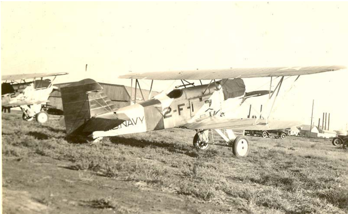
Above and following, four views of VF-2 "Fighting Two" aircraft based at NAS San Diego. Lack of arrestor gear indicates these are earlier land-based planes. The Boeing FB-1 (above), the Navy version of the Army PW-9, was powered by a 435 hp Curtiss D-12 "Conqueror" engine. With a top speed of speed of 159 mph, the FB-1 was slightly faster than the F6C-2 (below) powered by the same engine. Note VF-2 emblem beneath exhaust stacks. Markings designate number 5 aircraft of Fighting Squadron 2, prior to its nom de guerre as "The Fighting Chiefs." There appears to be a crowd on field, perhaps in conjunction with a Navy Day or other event now forgotten. As carrier aviation's first squadron, VF-2's 87-to-1 kill ratio during 1943-44 earned it the sobriquet, "hottest fighter squadron in the Pacific." Russ Gerow photo, Long Beach, c. 1928. R.T. Gerow Collection
