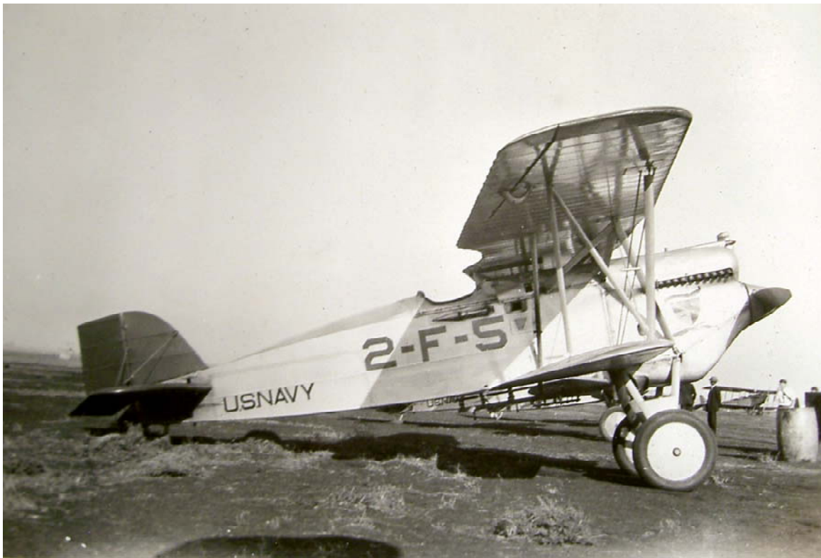
Above and following, four views of VF-2 "Fighting Two" aircraft based at NAS San Diego. Lack of arrestor gear indicates these are earlier land-based planes. The Boeing FB-1 (above), the Navy version of the Army PW-9, was powered by a 435 hp Curtiss D-12 "Conqueror" engine. With a top speed of speed of 159 mph, the FB-1 was slightly faster than the F6C-2 (below) powered by the same engine. Note VF-2 emblem beneath exhaust stacks. Markings designate number 5 aircraft of Fighting Squadron 2, prior to its nom de guerre as "The Fighting Chiefs." There appears to be a crowd on field, perhaps in conjunction with a Navy Day or other event now forgotten. As carrier aviation's first squadron, VF-2's 87-to-1 kill ratio during 1943-44 earned it the sobriquet, "hottest fighter squadron in the Pacific." Russ Gerow photo, Long Beach, c. 1928. R.T. Gerow Collection
