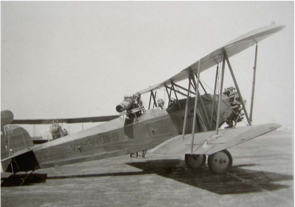
USNR Curtiss N2C-1 "Fledglings" of VN-13RD11 preparing to launch on a photo reconnaissance mission. Ponderous ring-mounted camera allowed observer to shoot verticals and obliques. Details of who these men are in this and the following photos have been lost with time. NRAB Long Beach, 1928. Russell T. Gerow Collection
